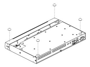
**Note:** To ensure adequate ventilation, allow at least 5.1 cm on each side, and 12.7cm at the back for power cord and cable clearance.
